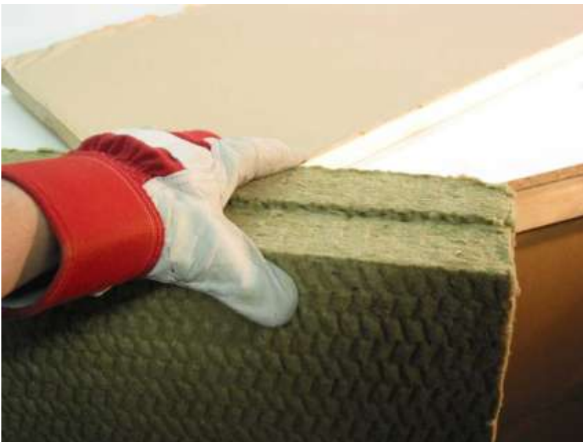
4" of 8 lbs. pcf density Rockwool: less rigid than 703, much heavier, tends to crumble, inexpensive, excellent acoustic properties.
