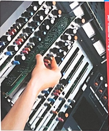
High-quality printed circuit components, modular assembly, speeds trouble-shooting and repair if needed.
